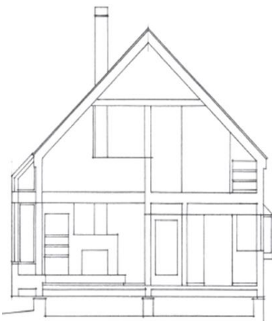
Here the section drawn with a single line weight.
